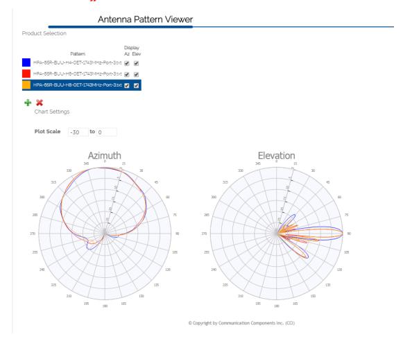
Figure 21 - Comparison of Port 3 on HPA-65R-BUU-H4, -H6 and -H8 Antennas (0° EDT, 1743 MHz)
