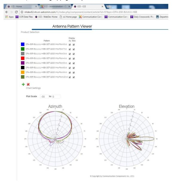
Figure 20 - All eight (8) High Band Ports on DPA-65R-BUUUU-H8B shown at 0° EDT, 1930 MHz
