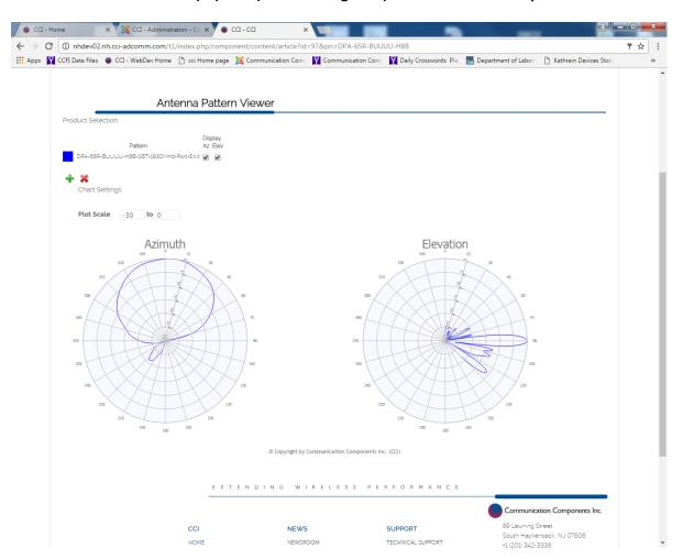
Figure 8 – Pattern for 0 Degrees EDT, at 1930 MHz for Port 5
